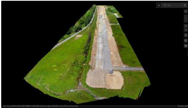
Barwick-LaFayette Airport Runway Reconstruction Project to increase its separation from a railroad in the Runway Object Free Area (ROFA) by 15 feet. UAS Mission flown by Demario Hall
