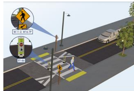
a: Raised Crosswalk
