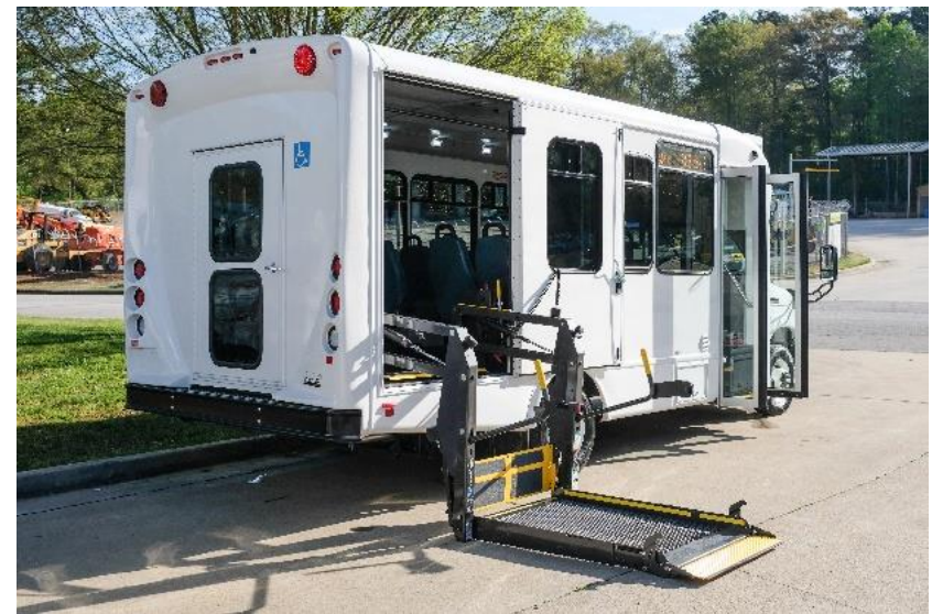
Figure 37. Wheelchair Lift Equipped Cutaway Bus
